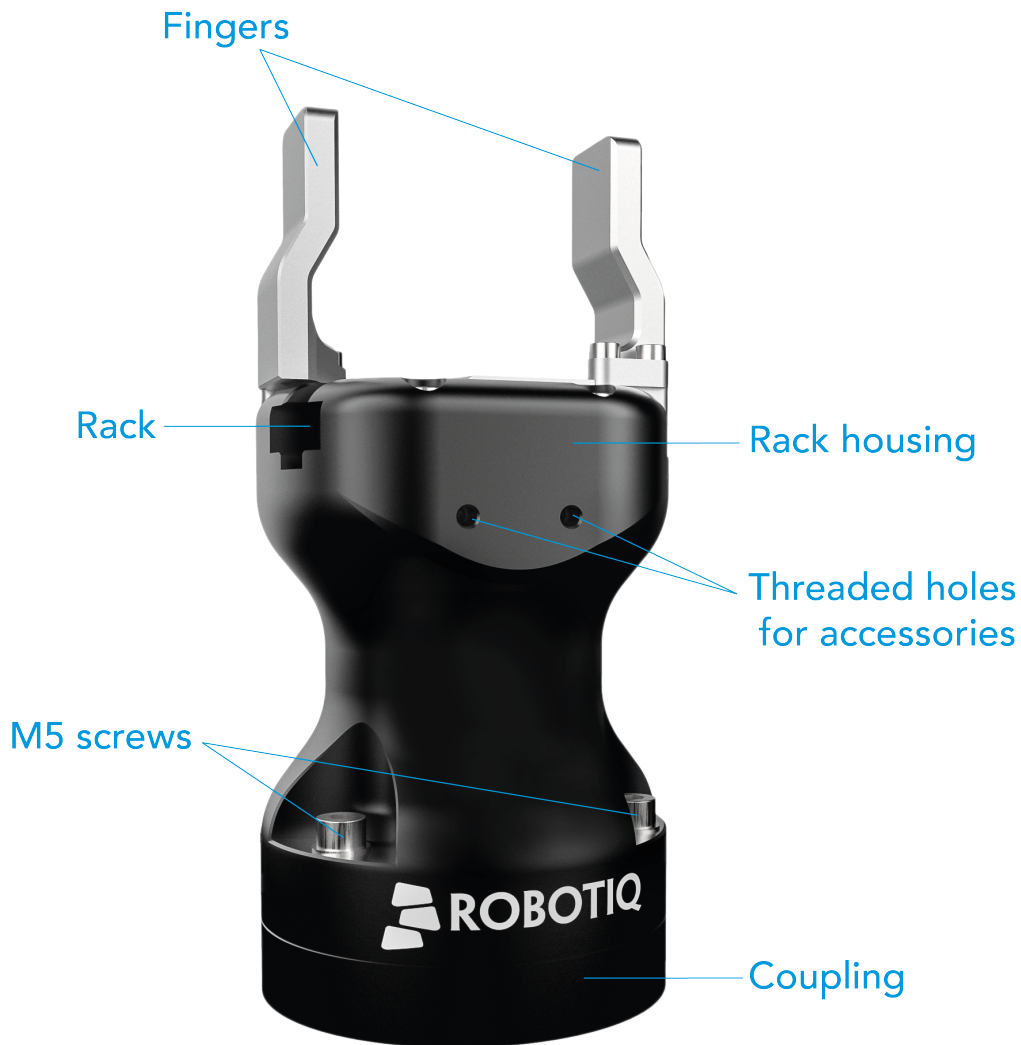
Fig. 1-1: Robotiq Hand-E gripper.
